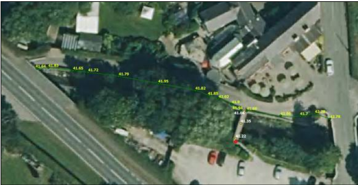
Figure 19: Surveyed levels of Wall on Left bank from A525 to Brookhouse Mill and footbridge deck levels
